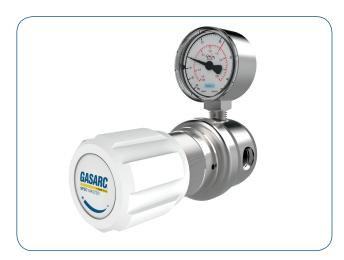
The Spec Master HPL600 Series single stage diaphragm line regulators are designed for secondary pressure gas control of non-corrosive or toxic, high purity gases up to grade 6.0 purity (99.9999%), on gas distribution systems.
